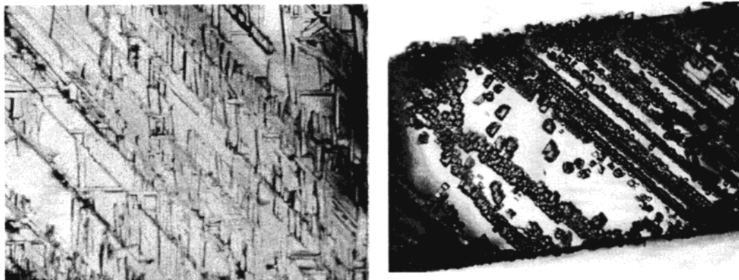
Figure 35. Photograph of benzoic acid (left) and p -nitroaniline (right) grown on (0\bar{1}0) faces of succinic acid. Nucleation initiates at the [101]_{SA} ledges, leading to oriented crystals decorating these ledge sites. The observed orientations are consistent with LDE-driven nucleation.
